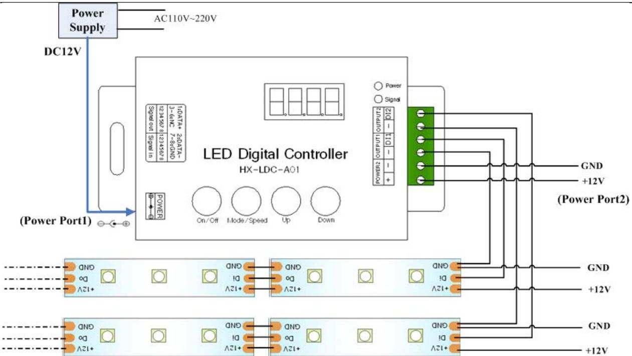
Application Circuit2, (Each controller can be individually powered, can also share power) Application of synchronization:
